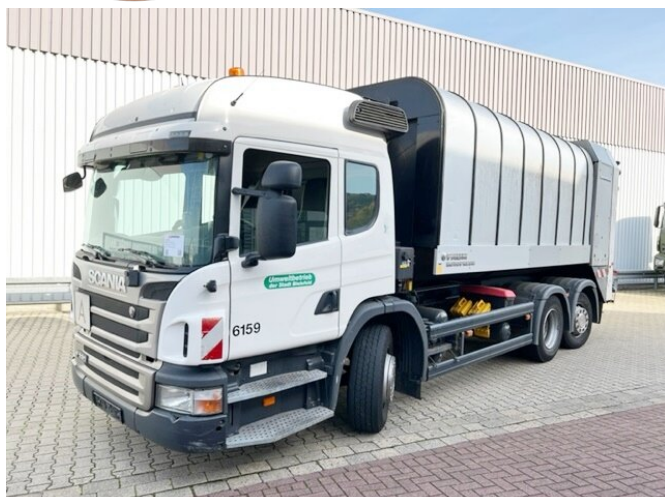
SCANIA (S) P320 6x2, Lenkachse, FAUN Rotopress 521
